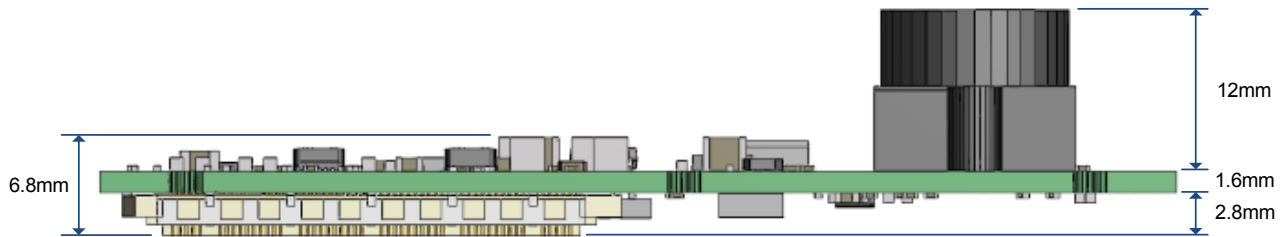
Figure 7-3 Side view of the TIM UP – 19k-S3-Spartan6
