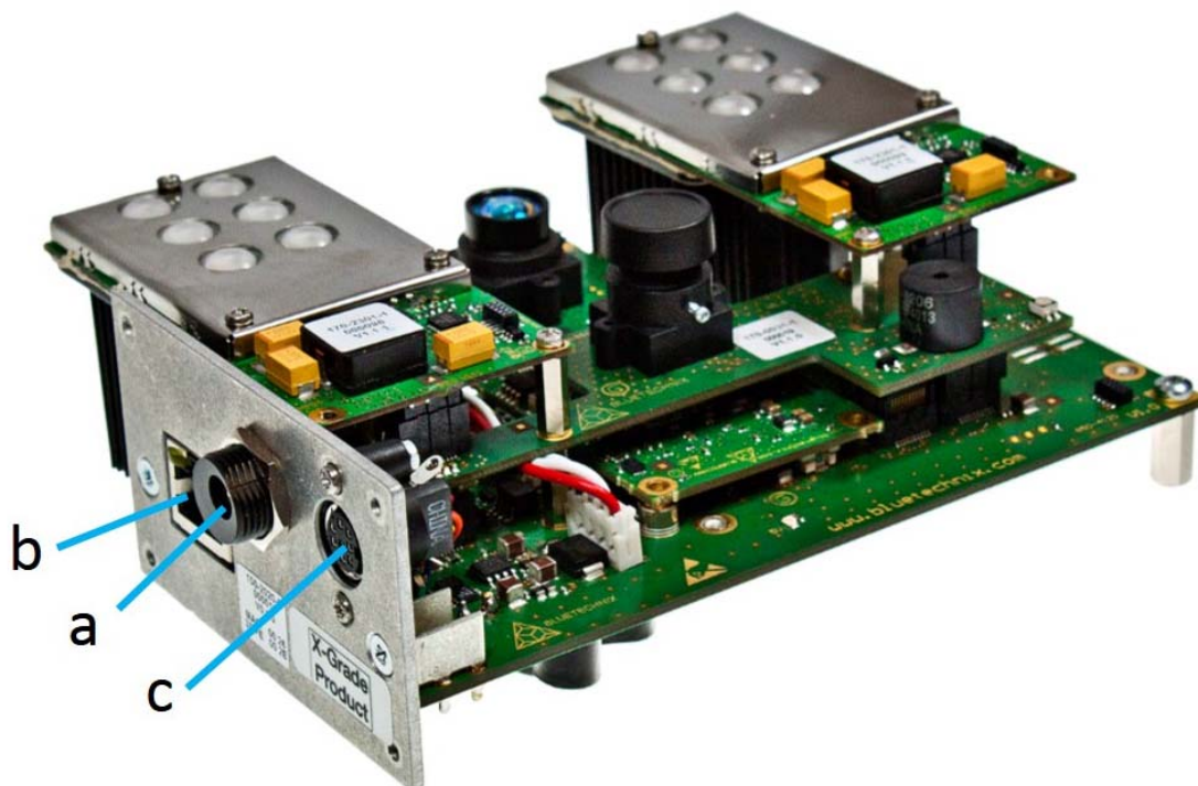
Figure 1-2: Sentis-ToF-P510 connector compartment screw positions
