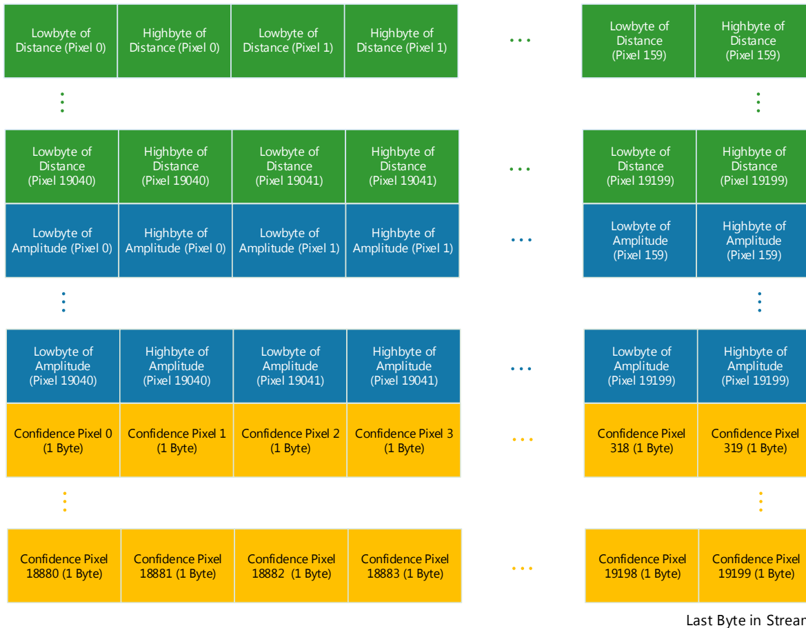
Figure 4-8: Data stream of Distances, Amplitudes, and Confidences
