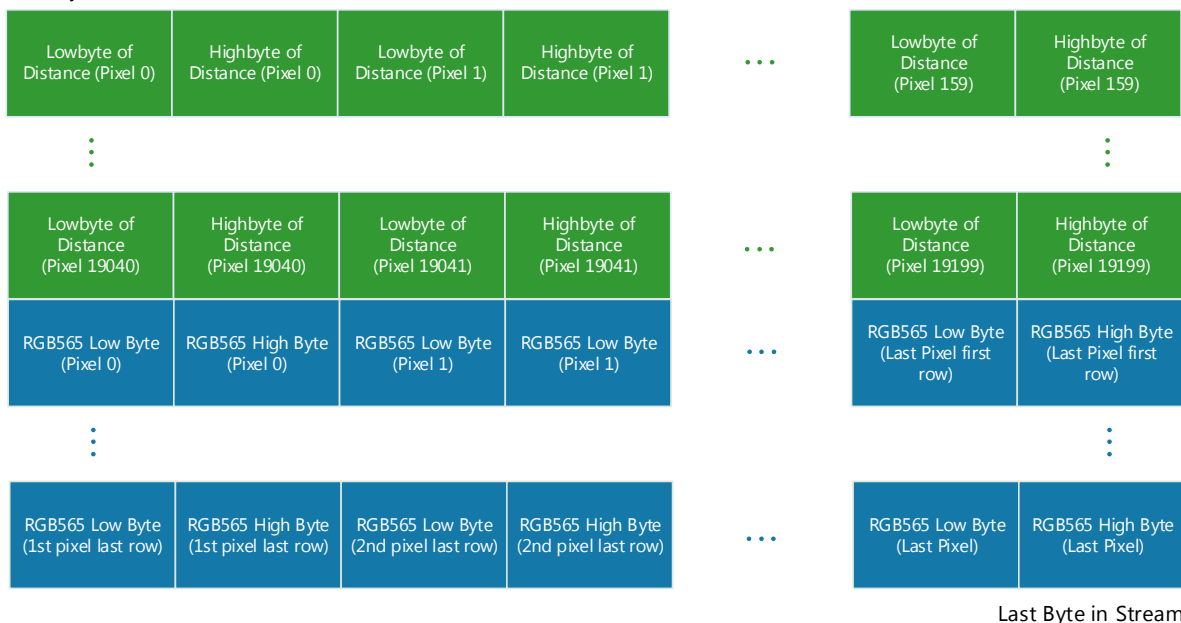
Figure 4-5: Data stream of distance and RGB565 data
