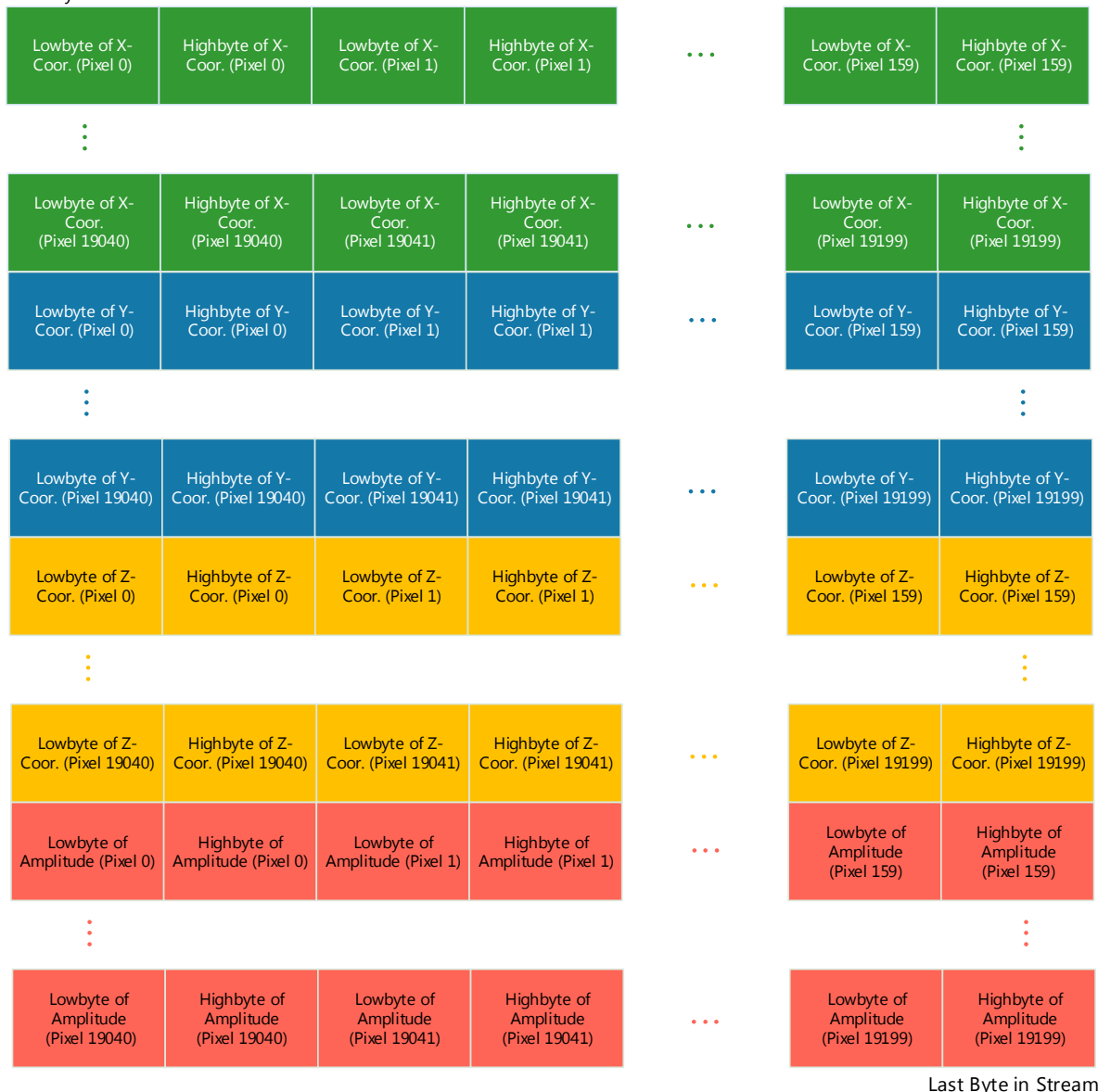
Figure 4-7: Data-stream of XYZ Point Cloud and Amplitude
