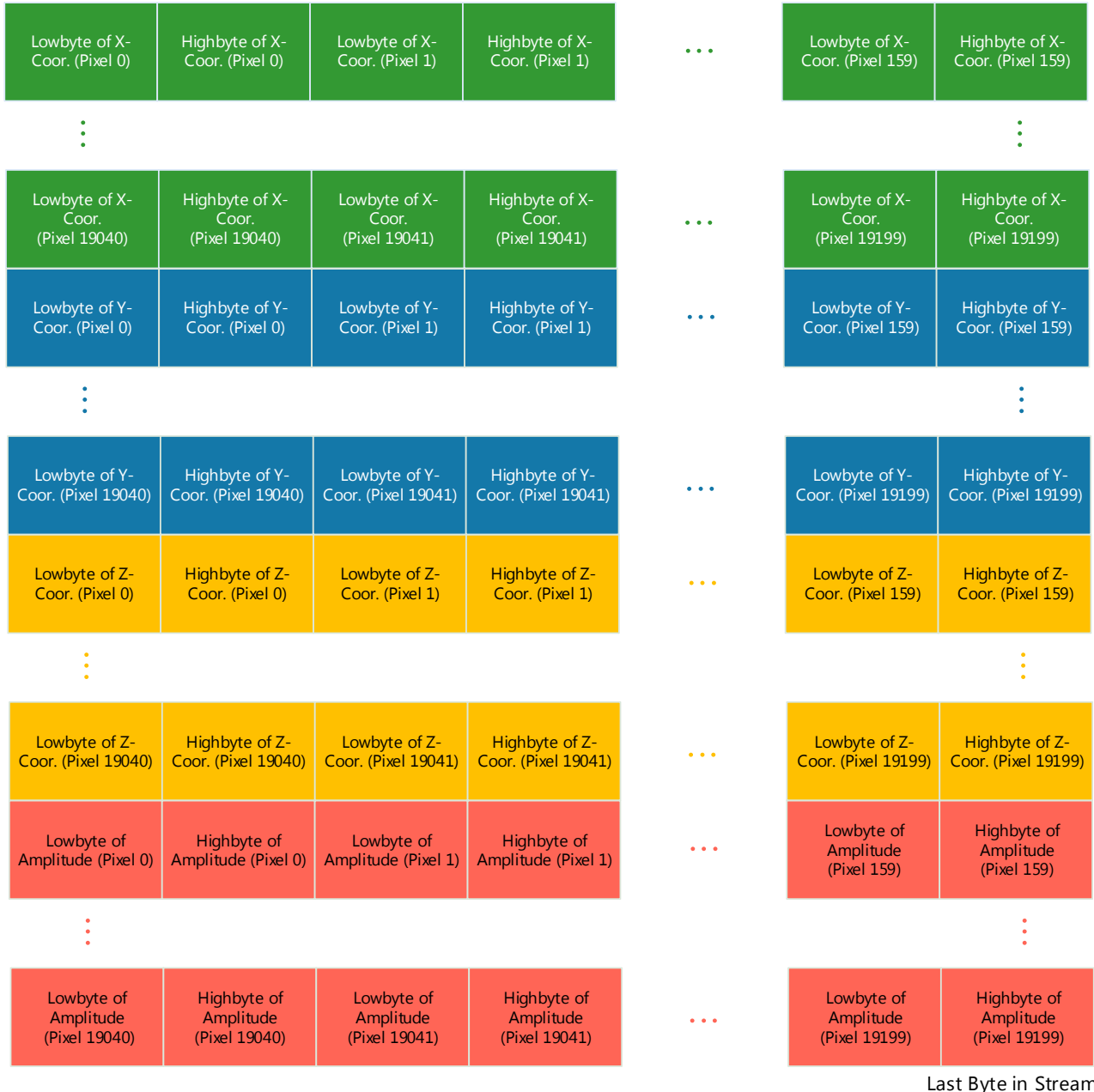
Figure 6-5: Data-stream of XYZ Point Cloud and Amplitude
