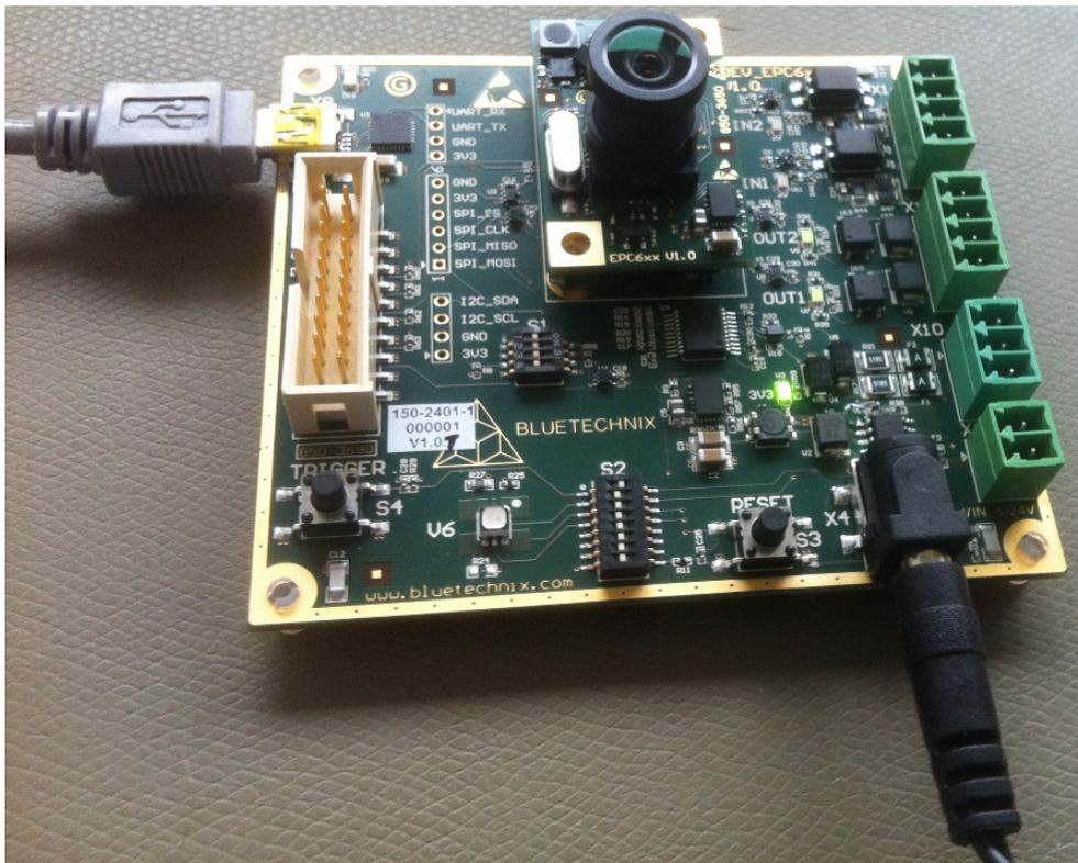
Figure 1-4: EPC6xx Dev. Board with connected EPC6xx ToF module, power supply and USB cable
