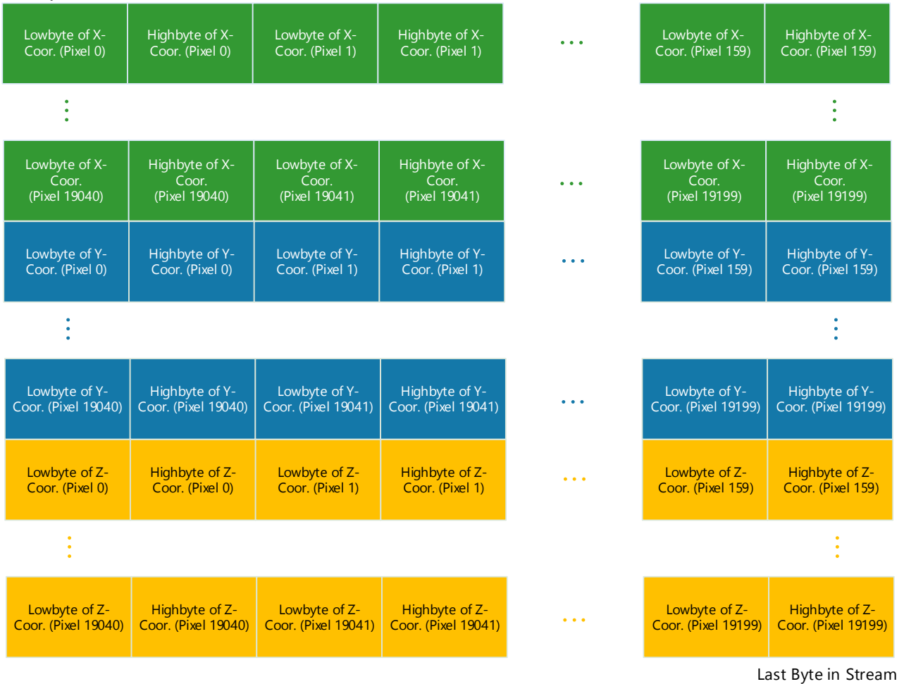
Figure 4-4: Data stream of XYZ Point Cloud
