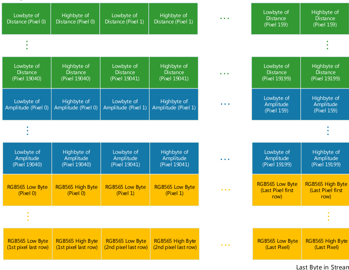
Figure 4-4: Data stream of Distance, Amplitude, RGB565 Color data
